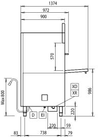
Cold Water inlet 1 (cleaning) Drain
